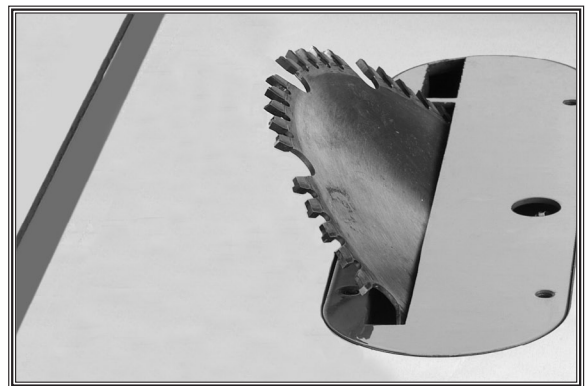
Figure 41. Blade tilted to 45^\circ (guard removed for photo clarity).
